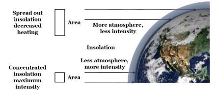
The effect of latitude – latitude sums up the effects of angle of incidence and Earth's shape and atmosphere
