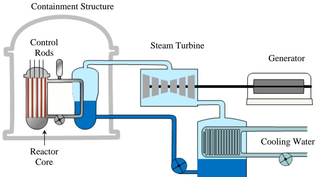
The water in the reactor core, the water in the steam system, and the cooling water are confined to three separated system to prevent escape of ionizing radiation
